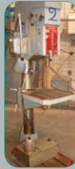
GRIMSTONE G35 Pillar Drill, 4mt spindle, speeds 90 - 1400rpm, power feeds and coolant. £2650
